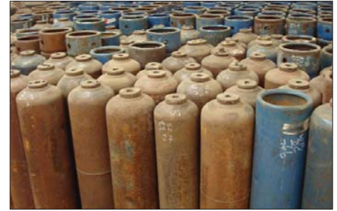
Acetylene cylinders that have been processed and are waiting to be sawed.
